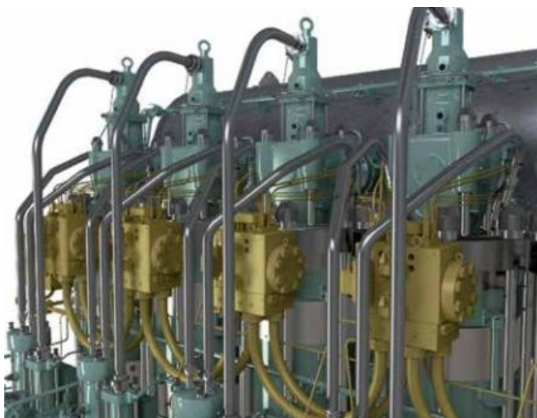
Fig. 6. New engine gas supply module.
