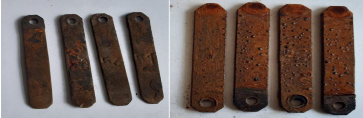
Fig. 4. Appearance of the samples after exposure in the pressure pipeline PS - 1
