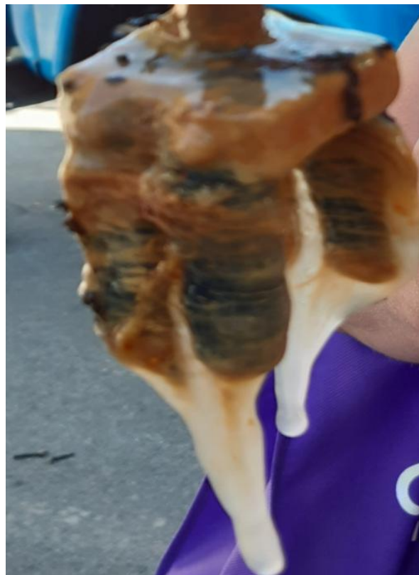
Fig. 5. General view of the samples after aging in the mix of groundwater and river waters
