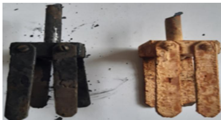
Fig. 1 Appearance of samples after exposure to groundwater wells
