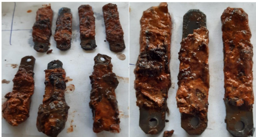
Fig. 3. Appearance of samples after exposure in the pressure pipeline PS-2
