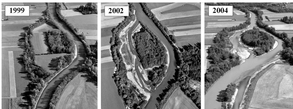
Figure 1. Drava River near Kleblach-Lind in the regulated state (1999) and development after initiation of a new side arm in 2002
