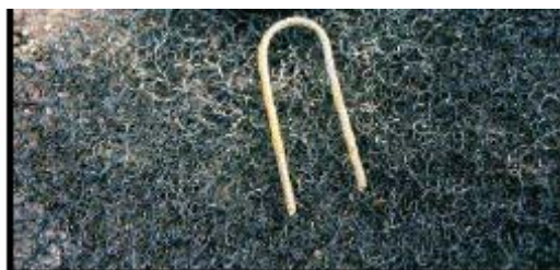
Photo 9. Metal look for fastening “Sekumat” in the soil
