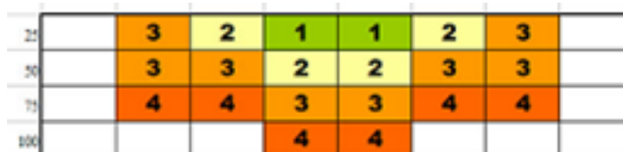
Fig 5. Horizontal Dam break model with time-step of 5 minutes. (100m deep. for 50m pixel DEM)
