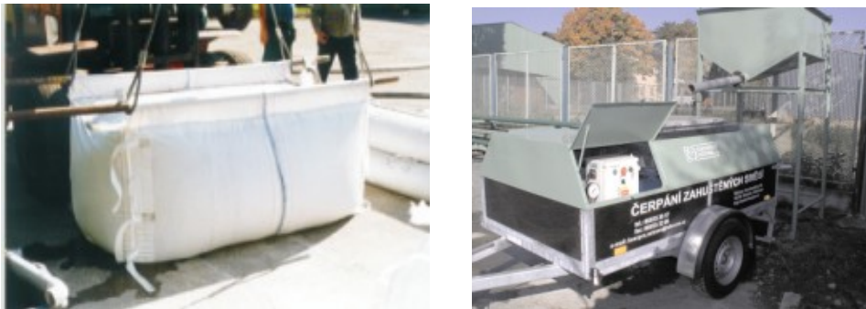
Fig. 3 Unit build bag 1x1x2 m and mobile screw pump KOEXPRO KTX 125/1
