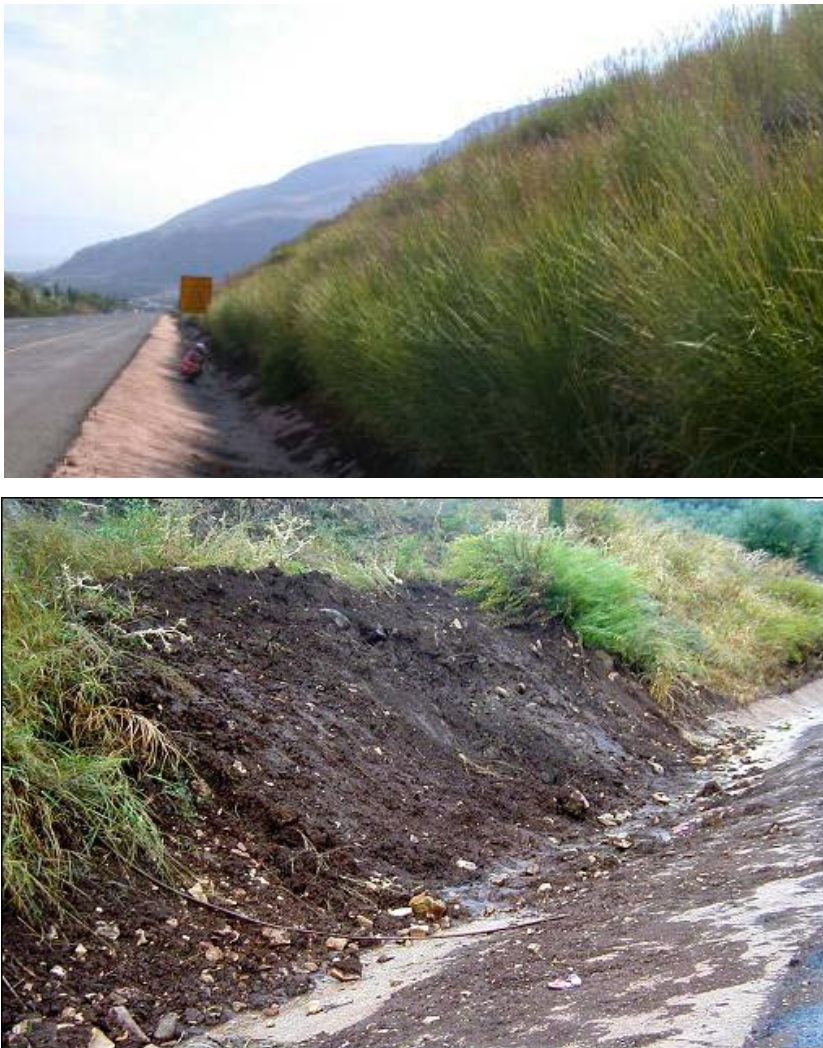
Fig. 2: The experiment at the Migdal coast site in October 2002: Top: a part of the slope with plants; Bottom: erosion in part of the control area (none planted).
