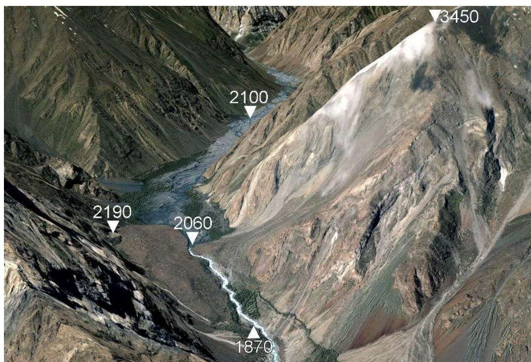
Fig. 10. Almost completely silted dammed lake in the Ak-Terek River valley. 3D Google Earth view
