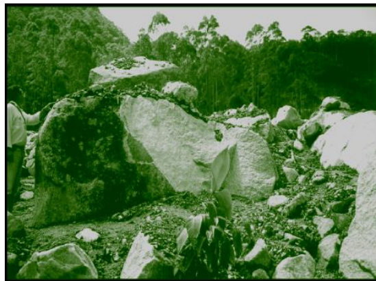
Fig. 3. Stony type debris flow with fragmented blocks of sienite (acid) rock increasing medium and small size grains content (M.F. Gramani)
