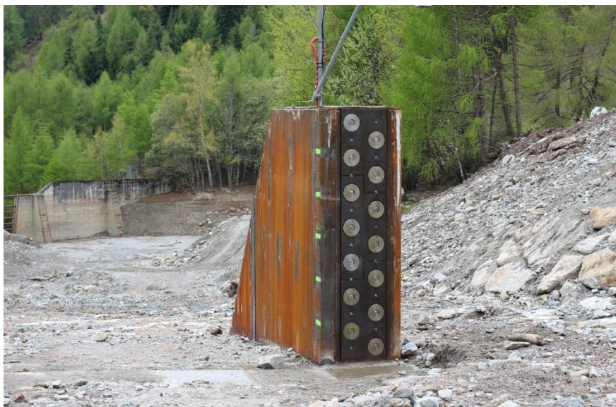
Fig. 1. Monitoring Barrier with fourteen load cells on the front
