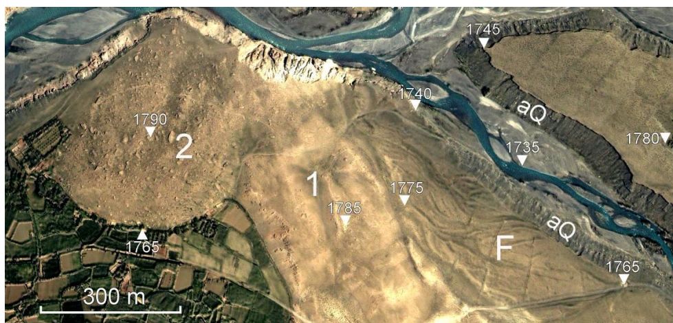
Fig. 3. Possible two generations of the Korgon rock avalanche body and evidence of the outburst flood from upstream. 1 – older generation of debris with smooth surface composed of finer material; 2 – younger generation with much coarser material; F – the specific landforms on the terrace surface left by outburst flood; aQ – fluvial deposits. Google Earth image
