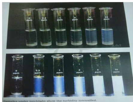
Samples under torchlight show the turbidity intensified.
